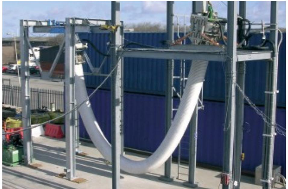
There are inherent hazards when handling cryogenics in a test environment. BPP-TECH therefore decided to employ a remote test management system, which would allow the engineers to conduct the test from the relative safety of a remote control cabin. The monitoring and control system used a data acquisition card as an interface between the sensors, and a central computer. The central computer was located in the same remote control cabin as the test engineers.
